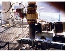
With over 12 years of continuous service in 1400° F (760° C), these 12-inch FCCU 3° stage cyclone catalyst separation valves have a remarkable life cycle cost when compared to other valve types.
