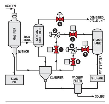
Proper blackwater treatment requires reliable valve performance under severe operating conditions.
