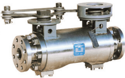
This 3-inch ASME 300 Class "one-of-a-kind" valve was built for a customer requiring customized fabrication and linkage. This 2-way valve, with piping entering the valve from the bottom, has two balls located within the valve body that open / close in an alternating fashion.
