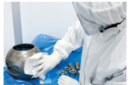
Stringent cleanroom processes for oxygen cleaning will effectively prepare parts for an oxygen-enriched environment.
