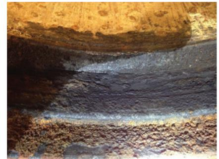
*Material loss in the seat pocket was caused by galvanic corrosion, allowing leakage around the valve seats.*
