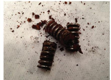
*Fine silt packed the coiled spring pockets preventing free motion and an effective seal.*
