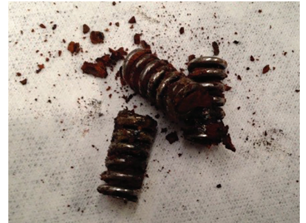
Fine silt packed the coiled spring pockets preventing free motion and an effective seal
