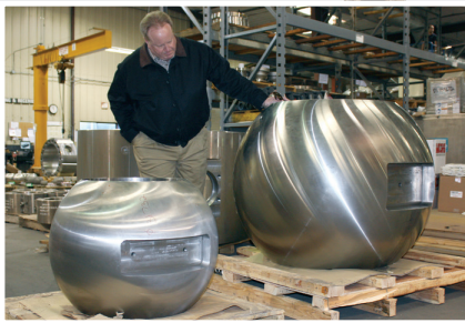
Many design considerations are needed for each valve component before simply enlarging a smaller size valve. For example, this 36-inch bore is considerably larger compared to the 24-inch ball, while the stem slots have different ratios due to performance requirements.
