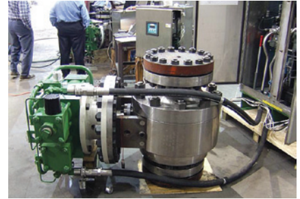
10-inch MOGAS valve / REXA electraulic actuator during testing.
