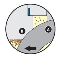
Integral seat designs do not allow bi-directional shutoff without a downstream check valve to prevent back pressure.
