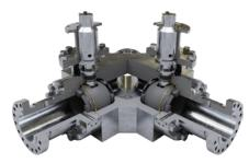
The MOGAS y-pattern valve provides the optimal solution for combining process functions, reducing required space, and diverting or isolating flow within a single valve body. Metal-to-metal sealing gives dependable, repeatable isolation in high temperature, high pressure and solids laden process streams.
