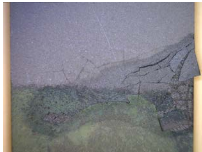
Figure 3: Thermally induced cracks on a n-TiO 2 /Alloy 20 coupon.
