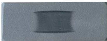
Figure 8: Photograph of a n-TiO 2 coating sample following abrasion test.
