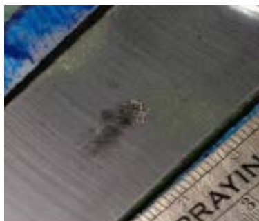
Figure 7: Photograph of a n-TiO 2 coating sample following impact test.
