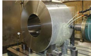
4. Machining of end connection
