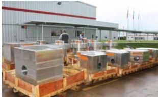
3. Rough machined material awaits final machining
