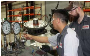
9. Pressure leak testing
