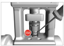
Use an air hose to clean debris from packing box before installing new packing rings.
