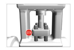
**13** Install and tighten nuts (15) evenly by alternating sides when tightening. Make sure the gland flange (07A) does not bind or drag on the stem (05).
