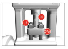
14 Cycle valve a couple times to ensure proper re-packing.
