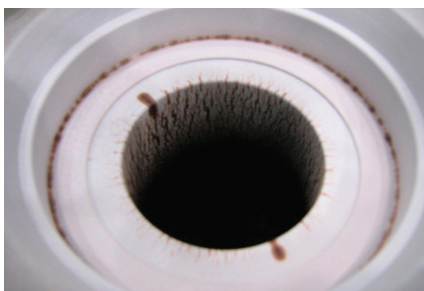
Dye penetrate check of thermal cracks to valve bore.
