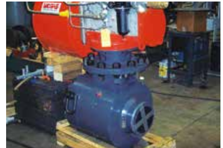
This boiler feed pump recirculation isolation valve was manufactured with high pressure hub ends with clamps to enable the customer to easily remove the valve for repair. This eliminates having to cut two very thick welds, rewelding and post weld heat treating.
