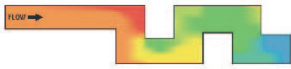
Figure 1. This CFD simulation in a control valve shows that by forcing process fluid to turn through a predetermined series of angles, kinetic energy is dissipated and velocity controlled.
